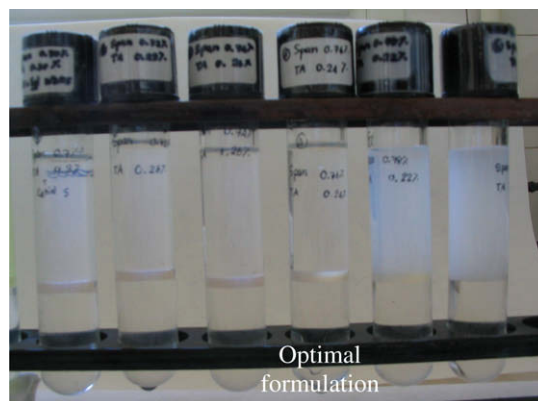
Fig. 1. Formulation scans of equilibrated (decylglucoside/sorbitan monolaurate)-dioctylcyclohexane-water systems at different (S/CoS) ratios. The three phase system with a microemulsion in equilibrium with equal quantities of oily phase and aqueous phase corresponds to optimum formulation.
